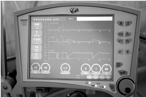
Fig.10. Pressure A/C (assisted/controlled)
